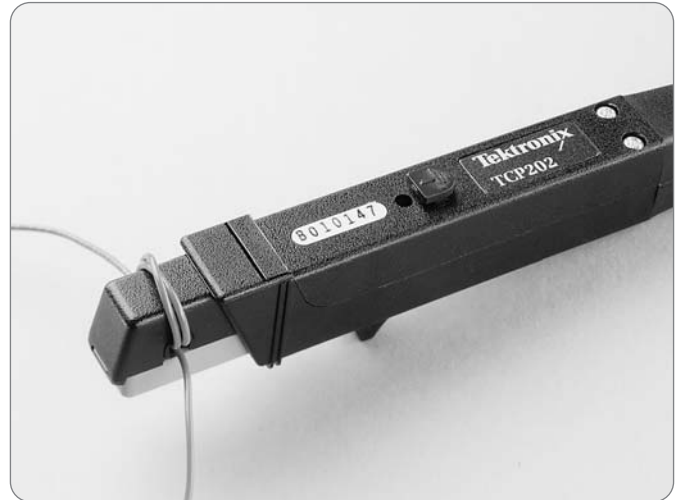
► Figure 2-8. An example of a split core AC current probe. Looping n turns of the conductor through the probe increases effective sensitivity n times.
