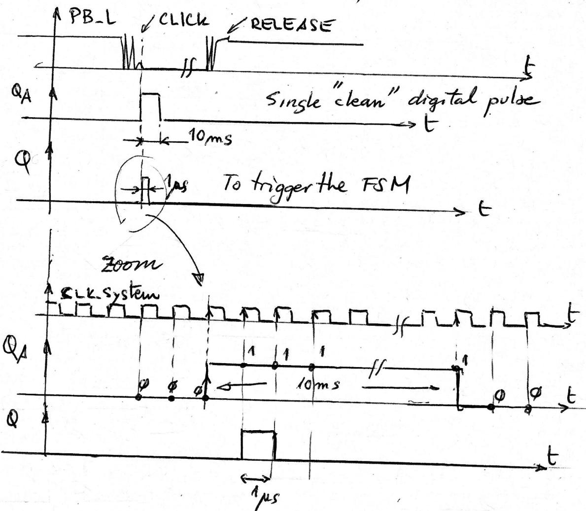
The CLK-Debouncer frequency (100Hz) is depending of the physical phenomena (Clicking a mechanical button)
