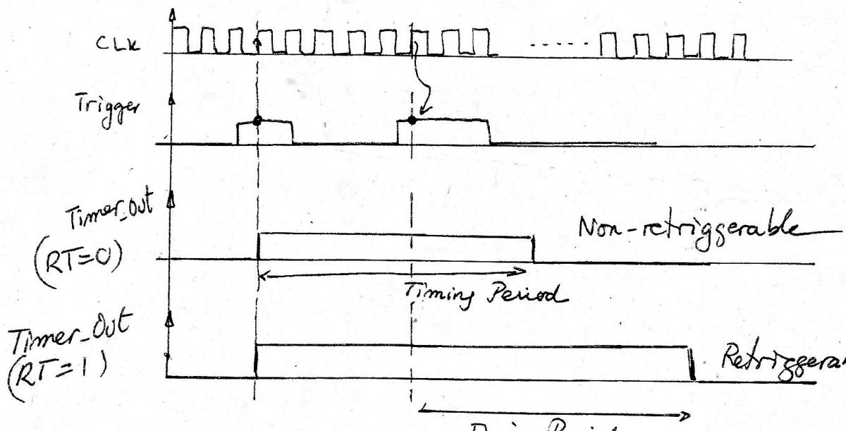
In the  $RT=1$  mode, see the 74LS122/123 classic chip, the timing period can be extended as desired because the timing period starts again every time that a Trigger signal is detected. This is the functionality of a "watch-dog" timer.
