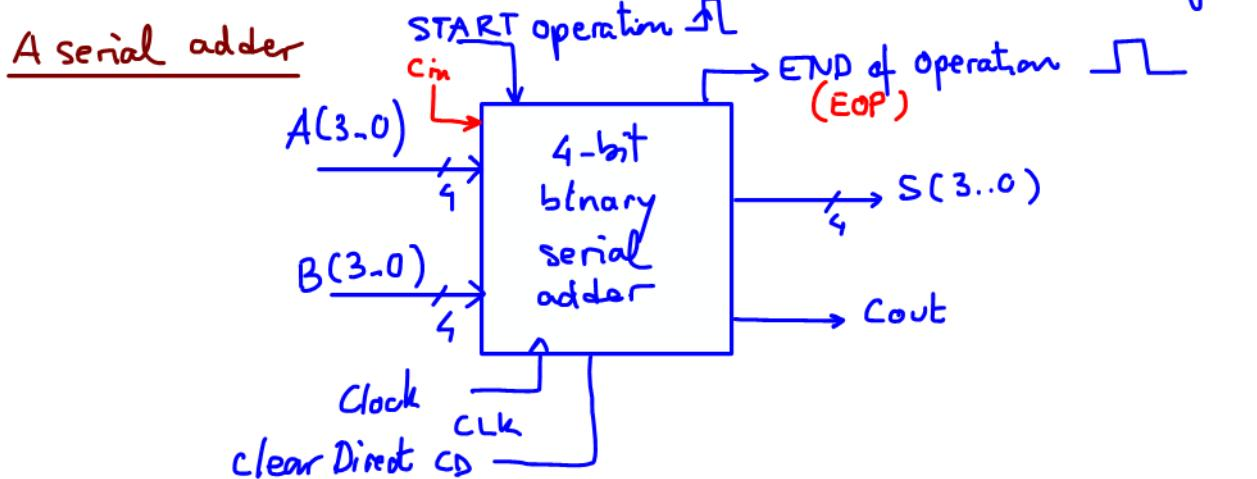
It will be planned for 4 bit operations, but can be easily inferred that it is enhanced in a single way to perform binary additions for larger numbers
